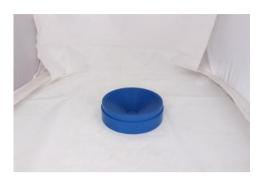
"Lab Smith" Flask holder is made of Silicon Rubber, to hold flasks from 10ml to 10000 ml, can withstand temperature up to  $280^{\circ}$  C.
