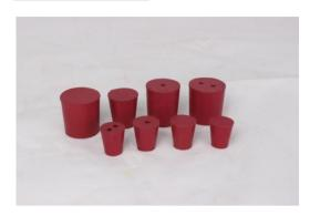
**"Lab Smith"** Rubber corks are made of natural rubber, shore hardness 45, density 1.13, temp. range -30°C to 70°C. Light weight & soft, it is resistant to dilute acid, alkalies, ammonia etc. In normal laboratory use.
