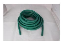
**"Lab Smith"** Pressure Rubber tubing is made of natural rubber, shore hardness 45, density 1.13, temperature range -30°C to 70°C light, flexible, for transferring gases, liquids. It is resistant to dilute.
