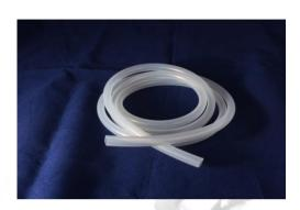
**"Lab Smith"** Silicon Rubber Tubing is Suitable for use over a temperature range of -50°C to 250°C, autoclavable, highly elastic. Resistant to strong alkalies, oils, bromine, carbon tetrachloride and toluene. Transparent tubing. Tubing is of medical grade, conforming to USP Class VI and also available in colors like: Blue and black.
