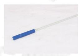
"Lab Smith" Rubber Policeman is made of Silicon rubber, to be used with glass or plastic rod of 5 mm Dia.
