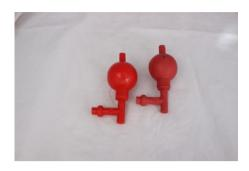
"Lab Smith" Pipette Filler has capacity of 50 ml, with a release valve to allow adjustment of liquid.
